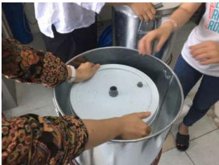
**Figure 6a: Main container and outside shell**
