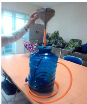
**Figure 2a: Rainwater collector (Test version)**
