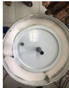
**Figure 6b: Insulated foam between main container and outside shell**
