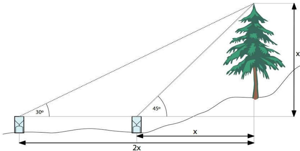
**Figure 1: Placement of a rain collector to minimize the influence of nearby objects [4]**
