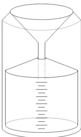
**Option 2: Tube-dip-in-water collector with pressure equilibration**
